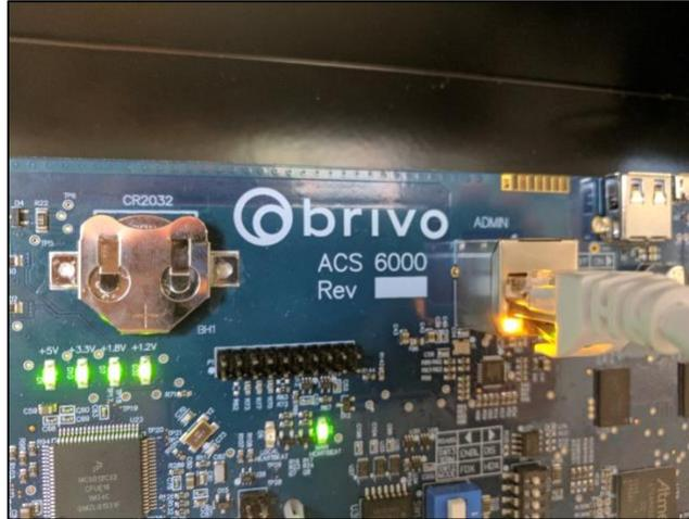
Figure 2. Connect Laptop to Admin Port on MAIN BOARD (Brivo Onsite panel)
