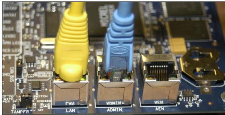
Figure 3. Connect Main Board to LAN (ACS5000-S panel)
